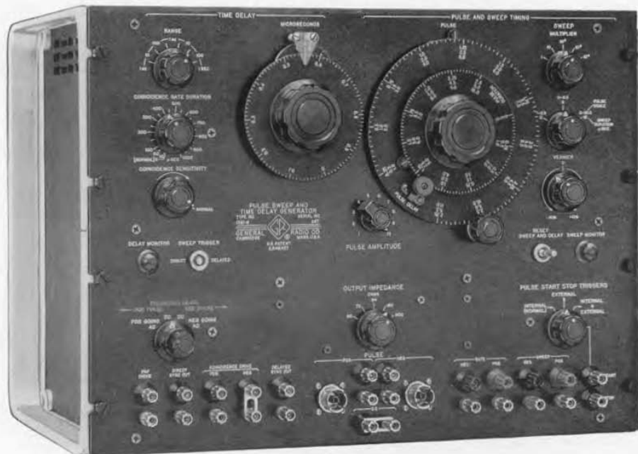
Figure 1. Panel view of the Pulse, Sweep, and Time-Delay Generator.
